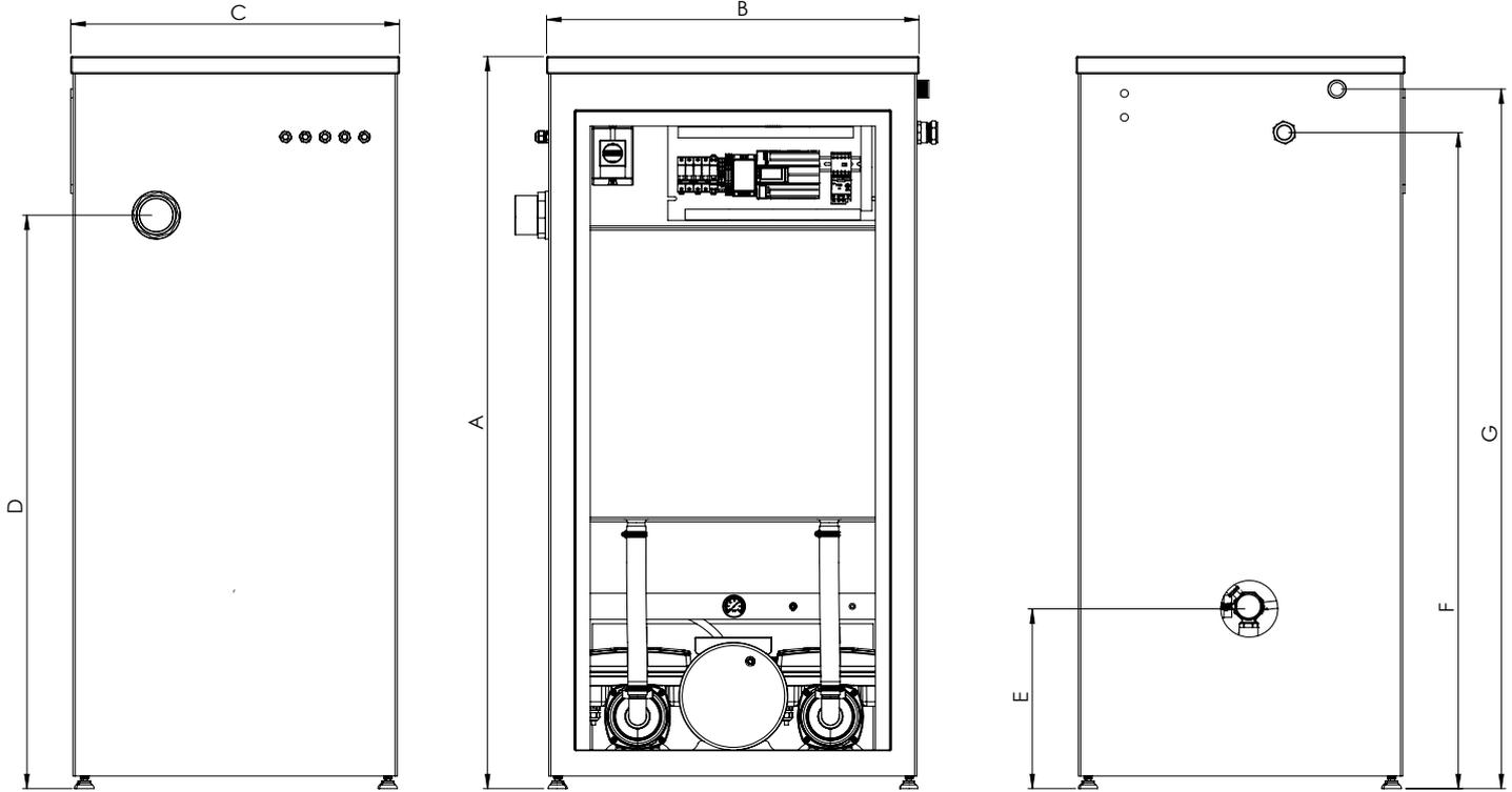
Unit must be installed at least 100mm away from a solid surface to enable the type 'AB' airbreak to function correctly at the back of the unit.
